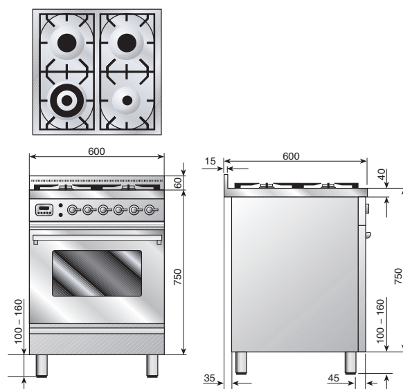
60cm Quadra 4 Burner Model PW60MP Total Electrical Load (Kw) 3.7 Total Gas 'NG' Consumption (Mj/h) 40
